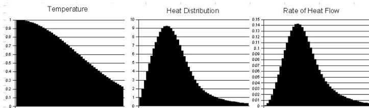
In the outer boreholes the temperatures fall well below the ground's ambient temperature so the graphs are mirror images of the injection graphs, but compressed because of the shorter period between the start of the
