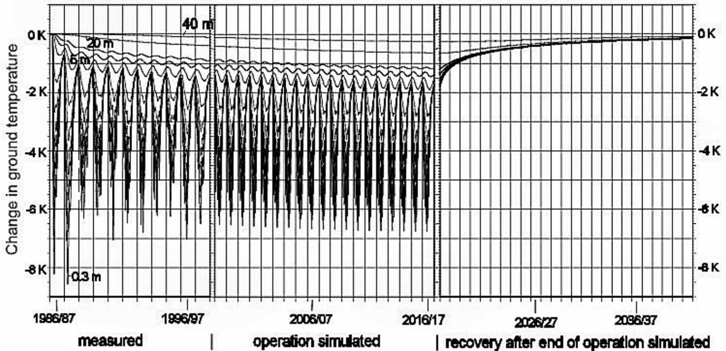
Changes in ground temperature at various distances from the BHE over many heating seasons, measurement and extrapolation (simulation) for the system in Elgg, Zurich, Switzerland.
