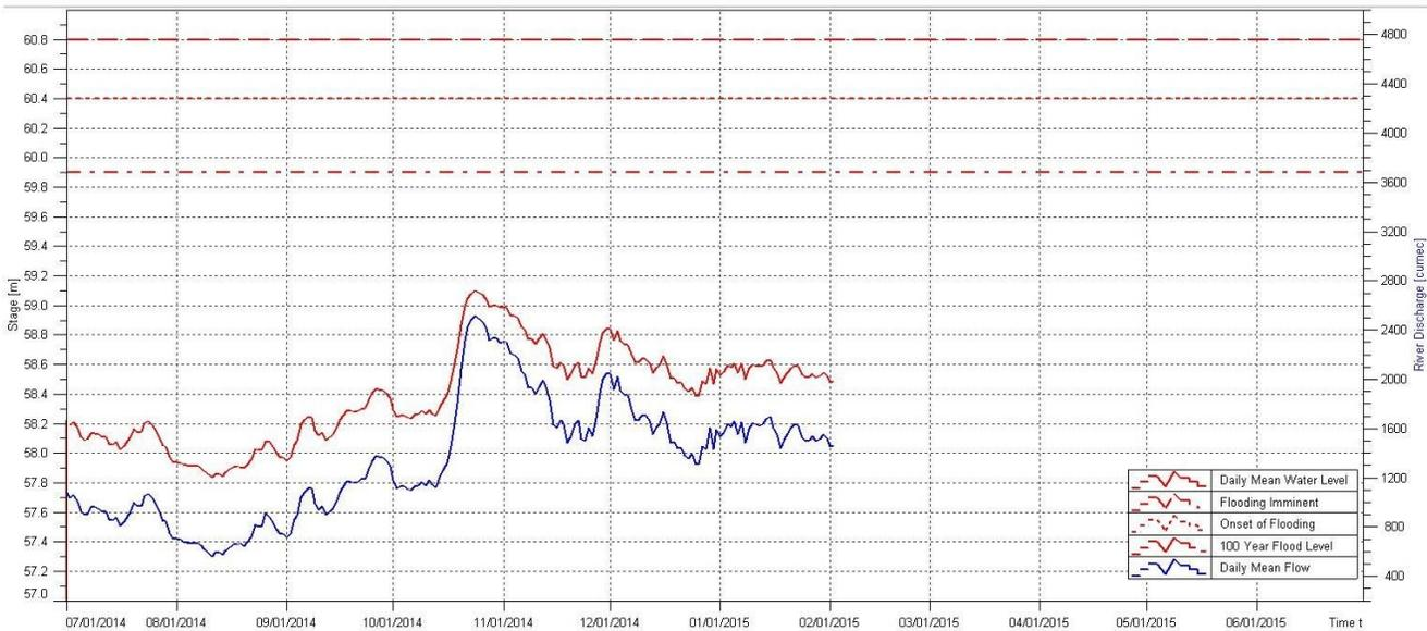
The bottom line (blue) shows the detail for the river flow at Britannia (downstream from Chats Falls). The plot above that line (red) shows the river height.
