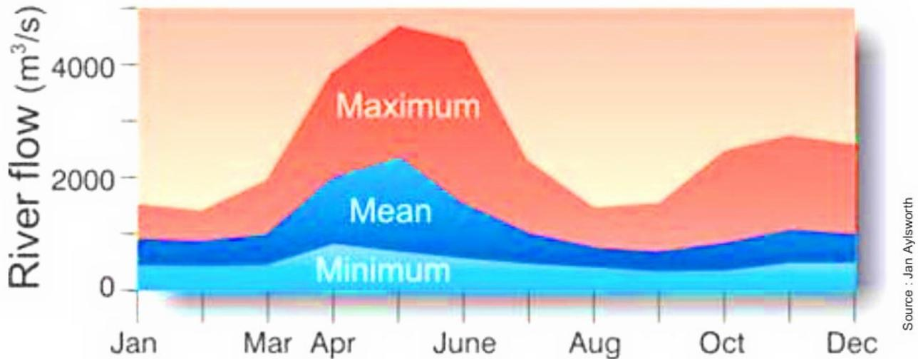
The Ottawa River has numerous dams that control its flow so it tends to have smaller variations than many other rivers but since all of the Ontario generators are run-of-the-river generators they cannot store the potential energy that is available during peak flow conditions. Given an external means of storing the energy their potential power output can thus be greatly increased. Note that the flow peaks in the Spring, coinciding with the period when the stores need to be recharged.
