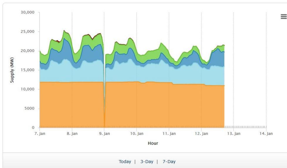
The orange colour represents the nuclear contribution which is relatively stable. Light blue represents the supply of electricity from all of the hydro stations that report to the IESO. Note that the output fluctuates according to the power demand, achieved by spilling some of the water through the spillways or by reducing the flow rate through the turbines which thus raises the pond water level (storing that
