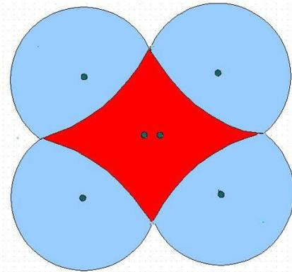
If the four outer boreholes are supplying the heat needed for domestic hot water (DHW) then the shape of the isotherm map remains almost constant throughout the year. In the summer the injected heat will “fill up the tank” by creating a thermal wave that will not reach the pincushion periphery until the fall. The temperature profile across the pincushion will change as the heat is injected but the shape of the perimeter will barely change at all.
