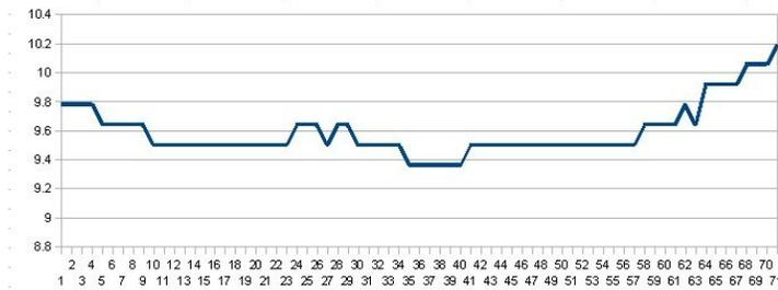
The increase started after an elapsed time of 58 days from the start of heat injection (the initial blips were caused by small amounts of heat that were injected directly into the blue hole during startup tests).
