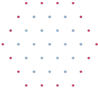
The above pattern shows the normal layout for the ground boreholes into which the heat is transferred. The depth of the boreholes is chosen to achieve the required storage capacity for the building in question. (Very small buildings may lack the outermost shell and very large ones may have one or two additional shells)
