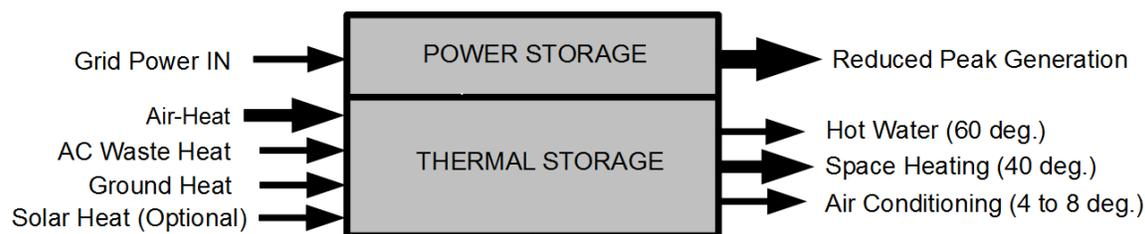
As with other grid power storage methods, the input power is converted into a storable form (thermal in this case) and this stored energy is used to reduce the need to generate power during peak demand periods. With most storage methods the output is less than the input but in this case the output is 2 to 4 times greater than the input because the associated thermal sources contribute exergy to the output. In effect a substantial amount of the thermal energy is converted into electricity.
