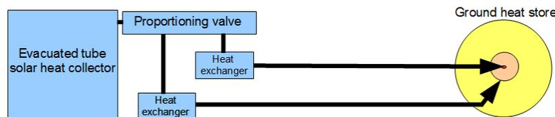
The drawing shows how such a system would work. Each house would have a small conventional electric hot water tank that would operate at a low power because its feed water would be preheated to very nearly the operating temperature via the input heat exchanger. Most of the thermal storage capacity is provided by the ground. The houses that have good solar exposure would have
