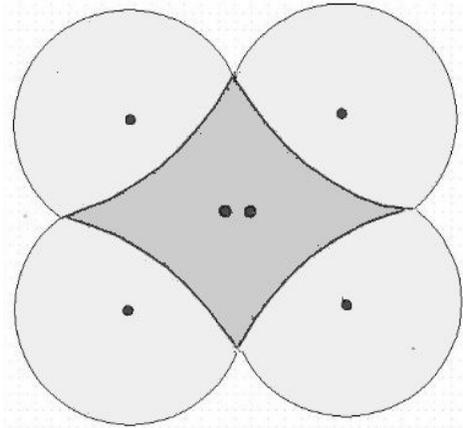
**Figure 3** Plan view of an AE heat storage field. Heat is injected into the two central boreholes and is extracted from the four outer boreholes. The central area is warm but the four outer areas (light grey) are chilled during the winter because of the extraction of heat. The field as a whole contains much more energy than the field of an equivalent GSHP .
