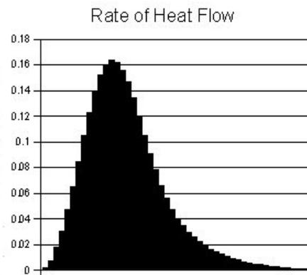
**Figure 2** Calculated rate of heat flow vs. distance from the borehole. For the central boreholes the heat is flowing away from the boreholes but for the outer boreholes as heat is extracted the flow direction is towards those boreholes. When these peaks overlap in the winter the primary heat flow is out of the central (warm) area to the extraction boreholes.
