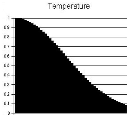
**Figure 1** Calculated temperature vs. distance from the borehole six months after the heat has been injected into the ground. Most of the heat remains within a distance of several meters from the injection point although the maximum temperature at the borehole has dropped substantially.
