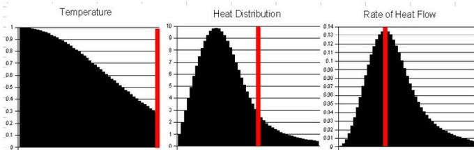
The outer boreholes for the demonstration system are located at an average distance of 4.5 metres from the center so the heat distribution curve indicates that very little heat will escape from the sides. About 5% of the heat will escape from the ends of this 20m deep store but for an AE-Street system, which will have much deeper boreholes, this loss will be much less than 1%.
