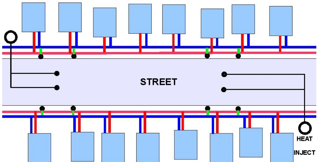
A pair of two inch pipes carries the warm and return water from the ground heat stores (under the street) to all of the homes. Only the central heat injection holes need to be located under the pavement and there can be as few as one heat store per 20 homes.
